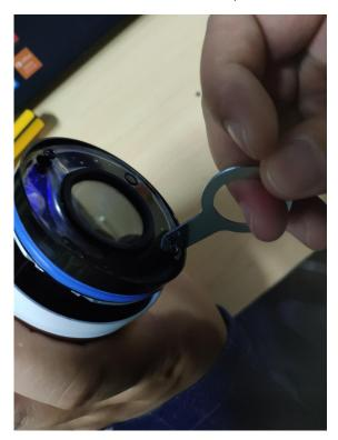
${\bf 2.}\ \ {\bf The\ lens\ is\ toward\ down\ ,\ then\ disassemble\ four\ screws\ in\ first\ board\ you\ have\ seen$
