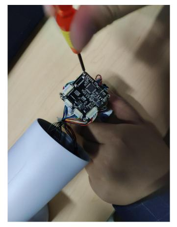
3. Then you will see second board which is main board. Take off four copper column And loose the WIFI connection cord
