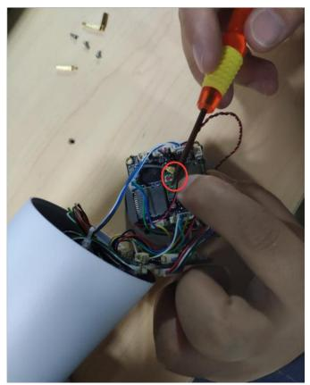
4. Pull out all cable on main board ( Suggest take a picture of wiring on main board in case of that you will forget when you put them back )
