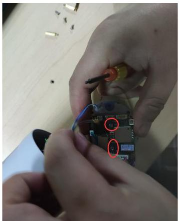
5. Take out the old board then replace it with the new Please ensure the sensor in red frame without any dust or fingerprint Then install two screws
