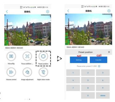
to the return position and continues to wait for the next tracking. The return position is 88<sup>th</sup> preset. please set 88<sup>th</sup> preset Call 97 for Turn on tracking, Setting method: [97]+[Call]; set 96 for turn off tracking, Setting method: [96]+[Set]
